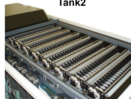
Top-view of an 8-tank customized processing solution to be used for gelatine paper coating
